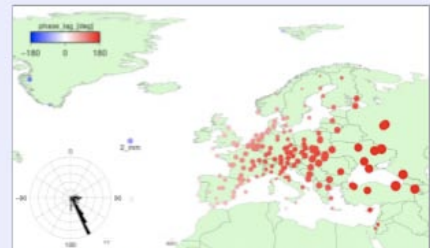
Fig.10/ GRACE solution: up component amplitude/phase distribution
